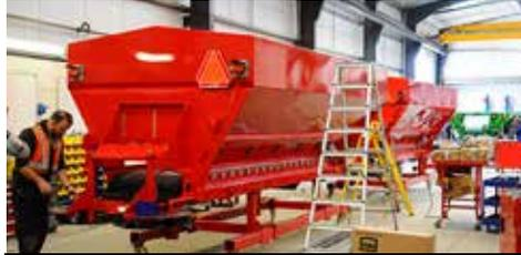
1st fix underway on the Fertiliser spreader assembly line
