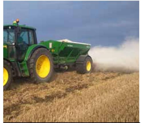
AS65 with Load cells, isobus rate controller spreading lime in the UK
