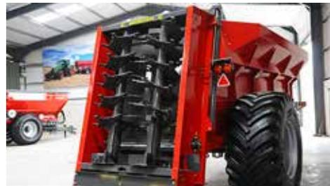
15 ton Twin Vertical Rear Discharge Spreader inside the factory for a recent factory tour
